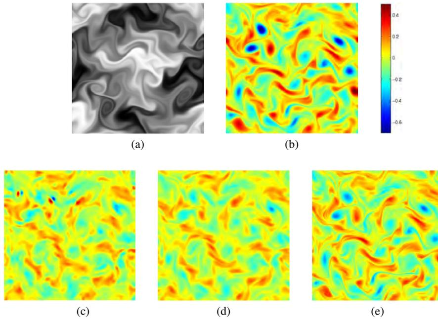
FIGURE 2. Synthetic 2D turbulent flow. (a) Example of scalar image of the sequence at given time  $k$ ; (b) Ground truth vorticity at time  $k$ ; (c) SLK vorticity estimate; (d) Mean estimate of vorticity with WENKF assimilation of SLK observation; (e) Mean estimate of vorticity with WETKF direct assimilation of image data.
