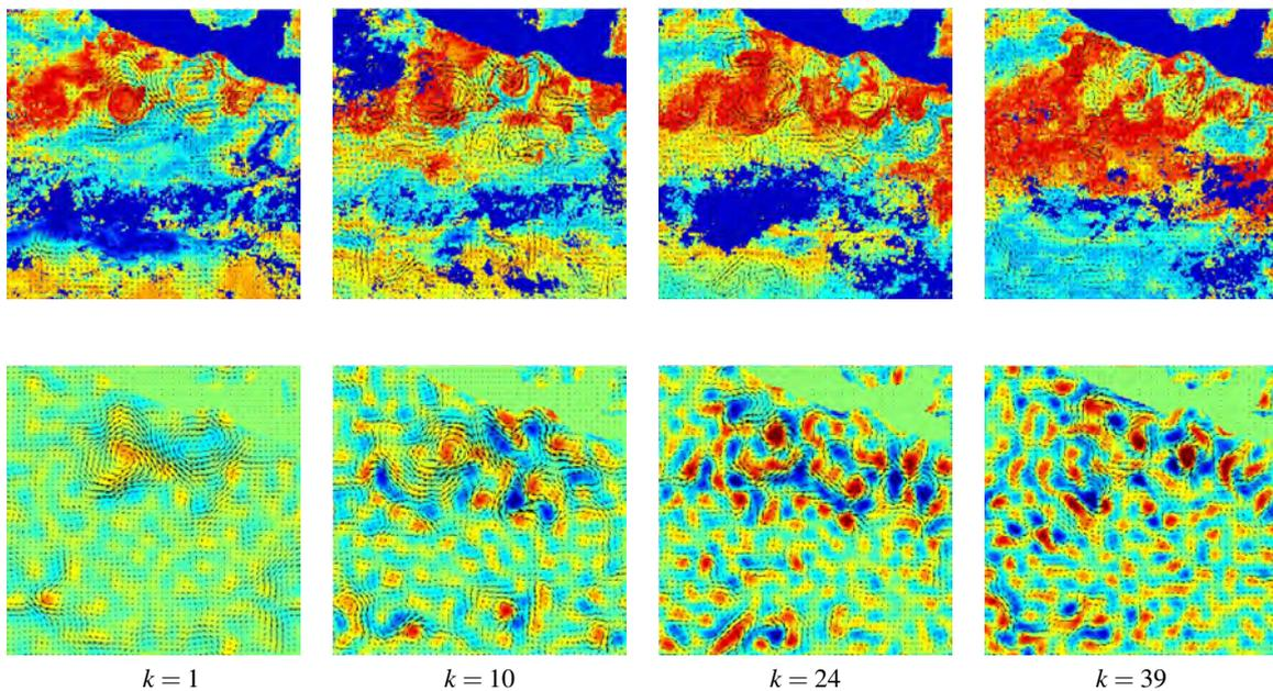
FIGURE 3. Real satellite sequence of SST (sea surface temperature) images. Dark blue regions indicate missing data due to the cloud cover or land regions. First row: SST images at different days  $k = 1, 10, 24, 39$  and estimated velocity fields with the WETKF assimilation of image data; Second row: Mean estimated vorticity with WETKF and associated velocity fields.
